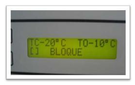
Prepare the cryostat by adjusting the chamber temperature at -20 °C and the specimen temperature between -10 °C and -20°C. The specimen temperature required for optimal cutting depend on each tissue. Select the desired tissue thickness (typically between 10 and 20  $\mu$ m).
