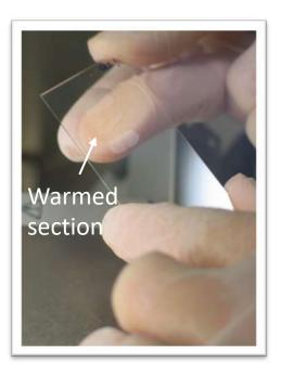
With both methods, inside the cryostat, place your finger on the nonconductive side back to the section to warm it. Wait until the section appears to be fully dry. You can put the slide back to the chamber and prepare another section.
