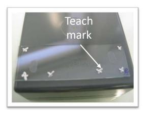
The slides must be scanned before matrix deposition. Teach marks are required for the correlation of the optical image with the sample in the instrument, it is therefore necessary to have teach marks that are visible both on the optical image and underneath the matrix layer in the camera optic. The easiest way is to spot at least three correction fluid (e.g. Tipp-Ex<sup>®</sup>) marks around the sample before taking the optical image.
