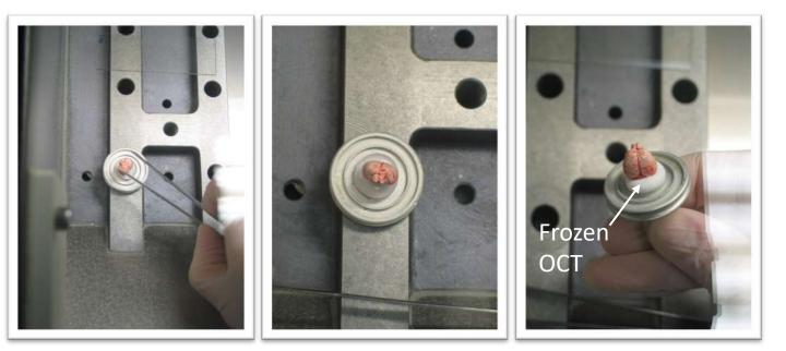
Promptly place the organ on the tissue holder and adjust its orientation before solidification of OCT. After a few minutes, OCT is totally frozen (and turns white) : the tissue is ready for sectioning.
