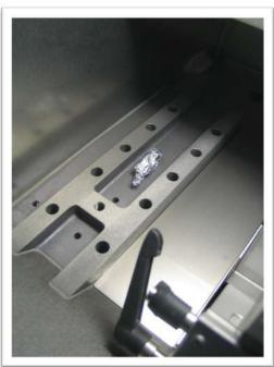
We recommend to transport the tissue on dry ice between the -80°C freezer and the cryostat. The tissue must be stored at chamber temperature (-20°C) for approximately 45 minutes before the start of cryosectioning. 5
