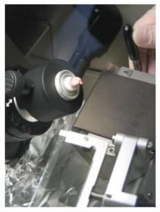
Wipe the cryostat blade with ethanol to remove contaminants. Insert the blade in the knife holder and lock the blade in place (right picture).
