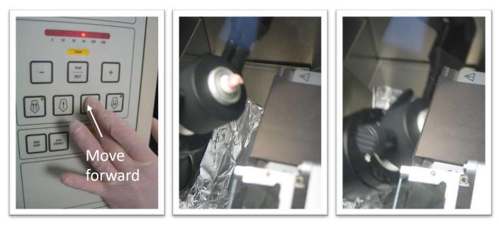
Move the anti-roll guide away from the knife. Move forward the specimen head using the four coarse feed keys (or any other command at your disposal depending on the instrument used) to bring the specimen close to the knife.
