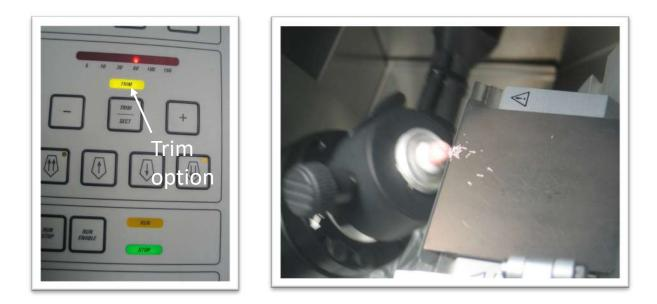
Rotate the handwheel to trim specimen down to the desired sectioning plane. You can use a higher section thickness (30-50  $\mu$ m) to go faster (use the trim option if available).
