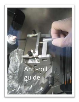
Place the anti-roll guide onto the blade. Carefully check the fine alignment of the anti-roll guide relative to knife edge.
