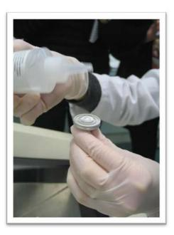
Deposit a drop of OCT on the tissue holder and place it in the chamber of the cryostat. Avoid any contact between OCT and regions of the tissue from which sections will be collected.
